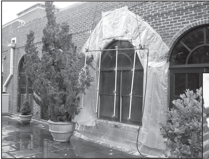
Figure 2 – View of water leakage testing in progress, isolating the window assembly.
