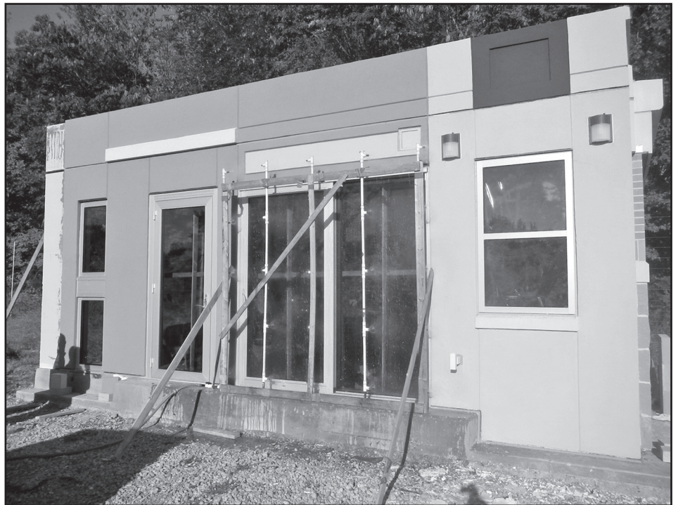
Figure 9 – View of large-scale off-site mock-up used to evaluate aesthetic issues in addition to water leakage performance testing.
