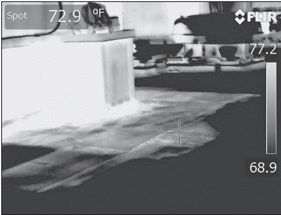
Figure 4 – View of wet region of roof insulation adjacent to the parapet wall.
