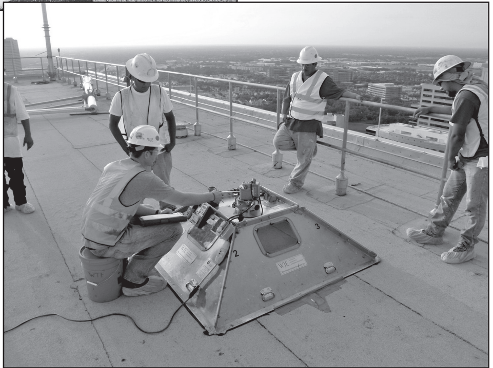
Figure 7 – View of roof uplift test in progress.
