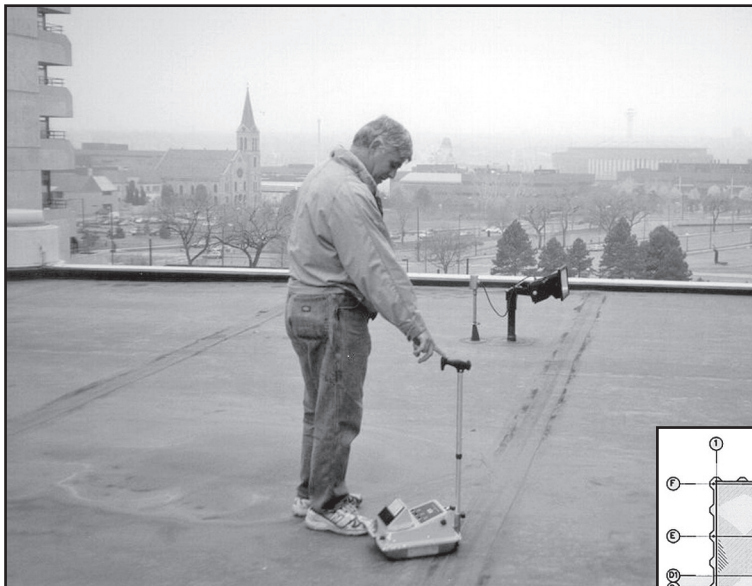
Figure 5 – View of nuclear meter survey and moisture map.
