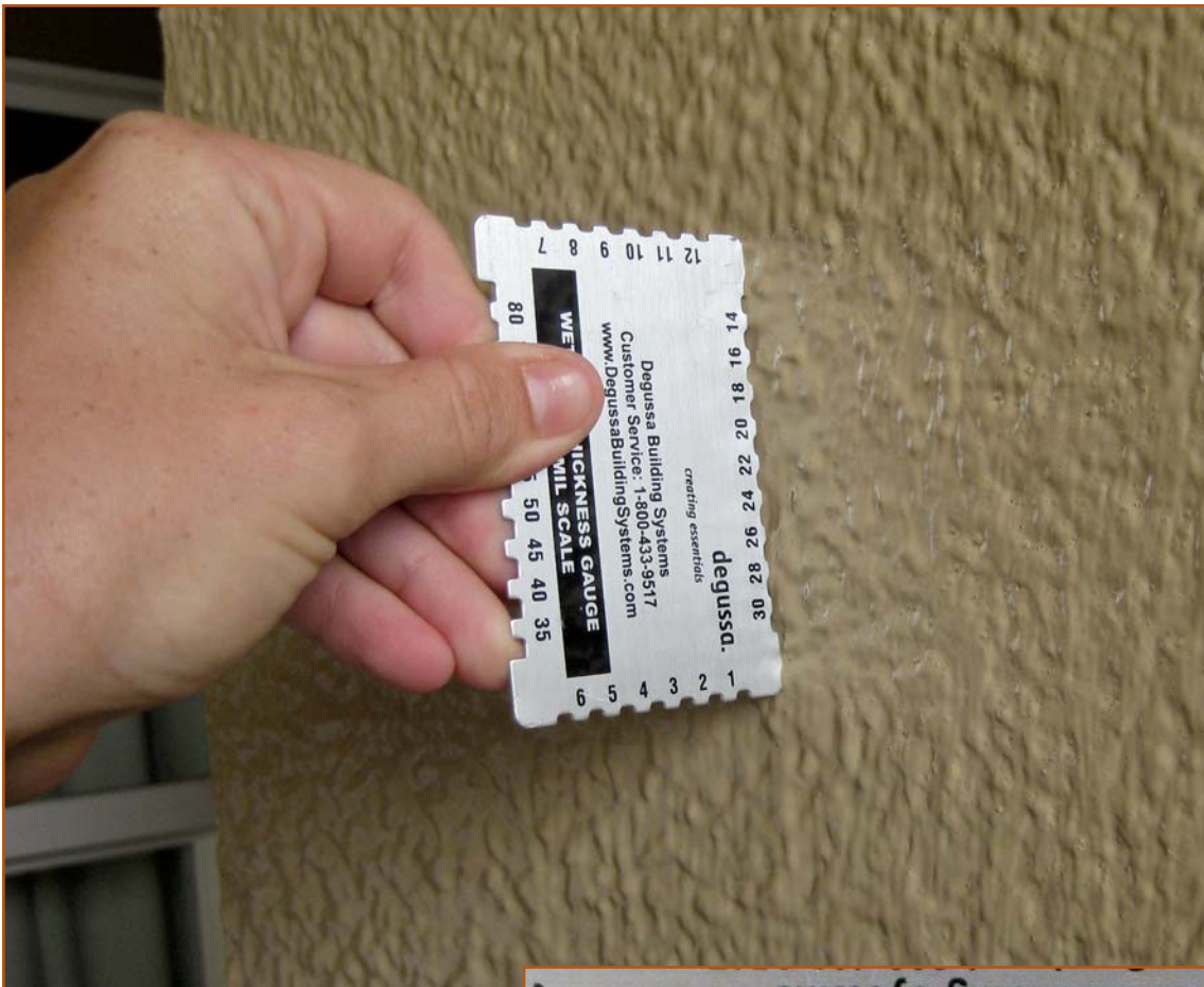
Figure 1 – A notched gauge used on a wall in the field immediately after application of an elastomeric coating.
