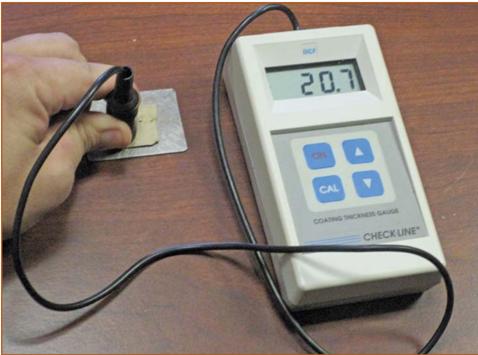
Figure 7 – A monopolar, magnetic induction device is used to determine the DFT of a coating sample removed from a wall area. On this particular project, a minimum of 16 DFT was required for warranty. This sample satisfied the requirements for the project.
