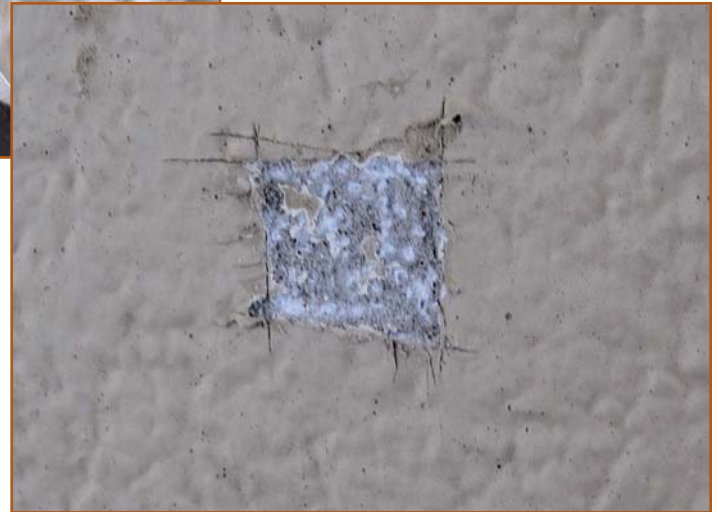
Figure 6 - The destructive method of removing a small sample of coating will require that the area be “touched up” after the DFT is measured.
