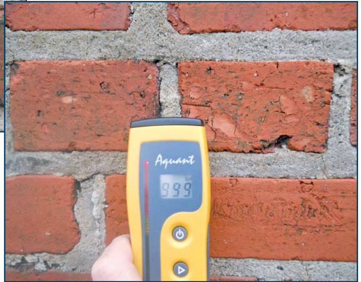
Photo 6 – High (red) reading on mortar.
