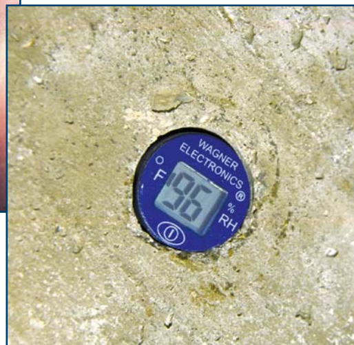
Photos 11A and 11B – Another relative humidity instrument uses probes that are inserted into a sleeve. The relative humidity is displayed on the top of the reader.
