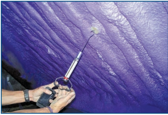
Figure 17 – Pull test for foam insulation.
