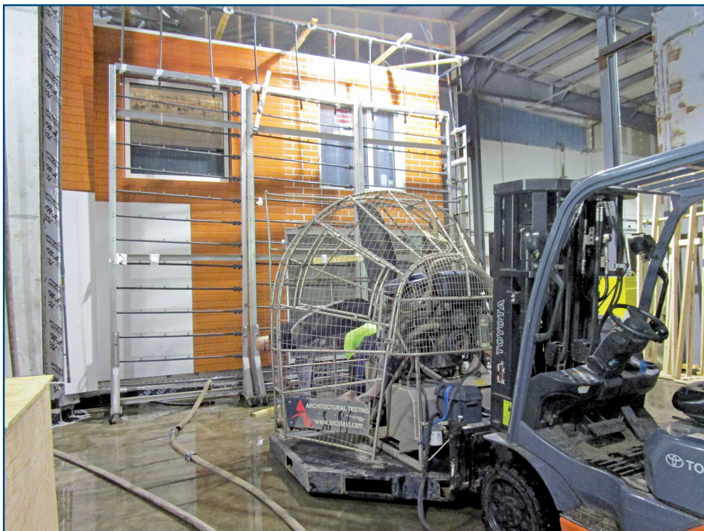
Figure 9 – Laboratory testing the panelized wall system.
