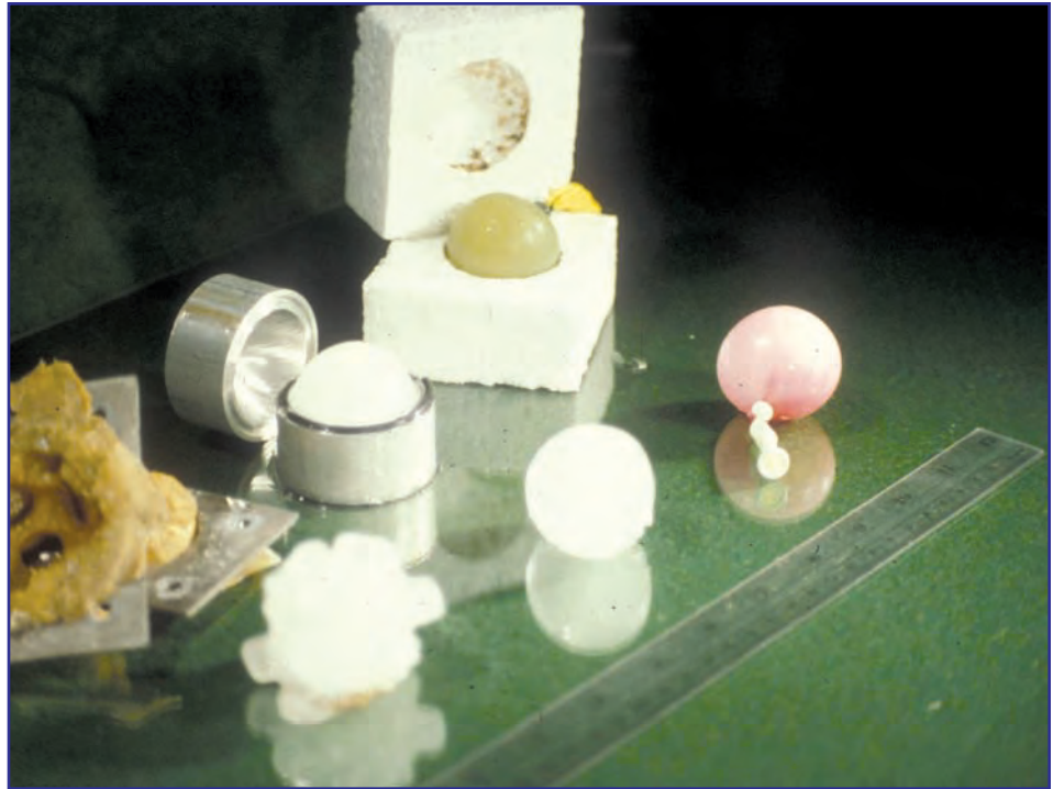
Figure 7: Ice-ball molds. Photo courtesy of Milton Smith, Texas Tech University.
