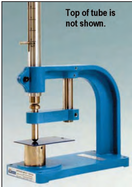
Figure 4 — Heavy-Duty Impact Tester PF-1120. Photo courtesy of BYK – Gardner, a member of the BYK Additives and Instruments Business Unit of Atlanta.
