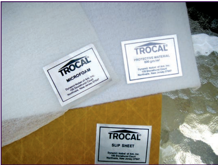
Figure 12: Various slip sheets have been used with plasticized PVC membranes.
