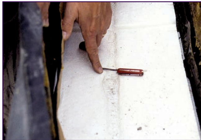
Figure 16: Cells of polystyrene foam have collapsed from solvent vapor attack.
