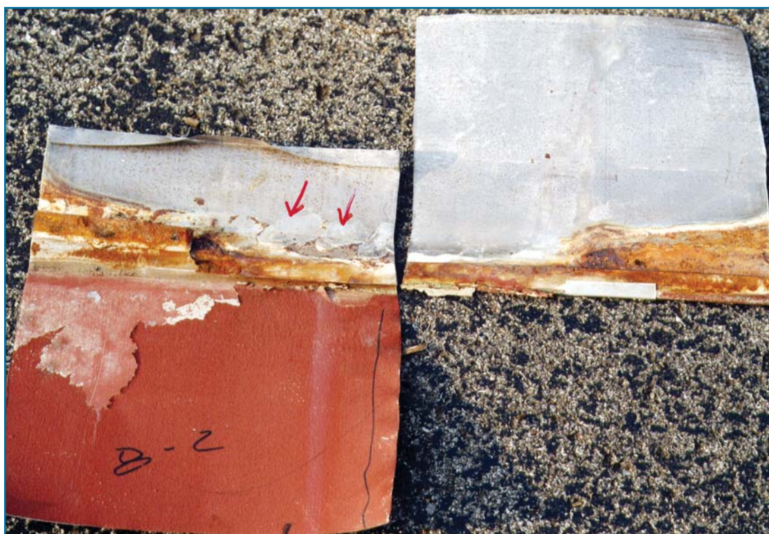
Figure 10: The left panel is the down-slope panel. The arrows indicate solder that was used to attach the lock-strip. Both sides of the lock-strip were very corroded. The right panel is the underside of the up-slope panel.
