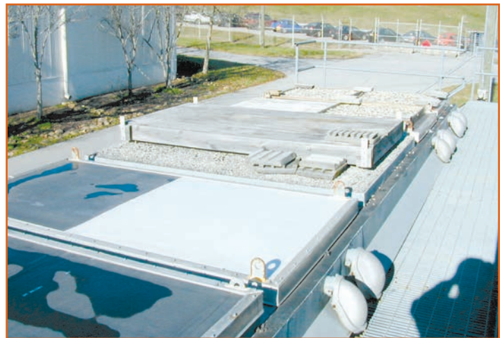
Figure 2: Test sections configured for the ballast test.
