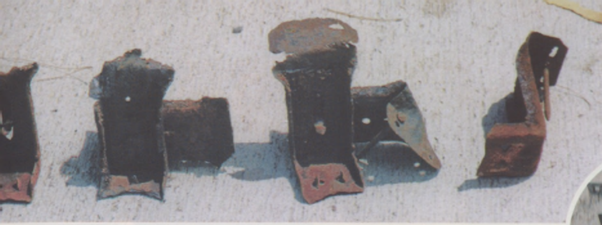
NEW (FACE-NAILED) SUB-PURLIN HANGER
