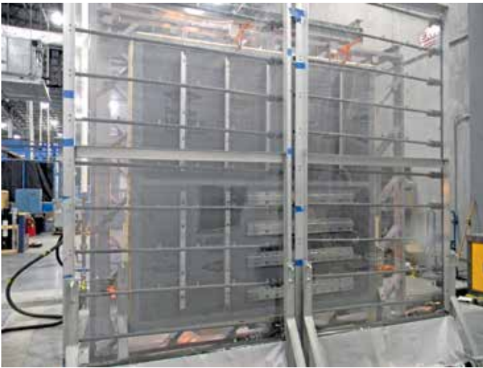
Figure 7. Wall shown in the test setup. Various girts are attached with different flashing configurations. A spray rack is in front of the wall.
