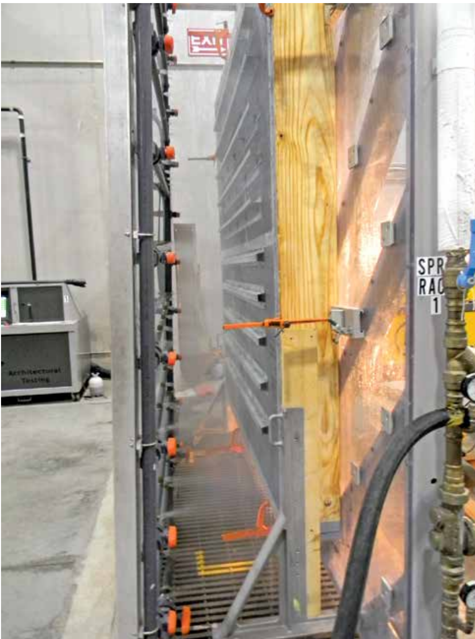
Figure 8. Side view of the wall during test. Water is seen coming out of various nozzles on the spray rack.
