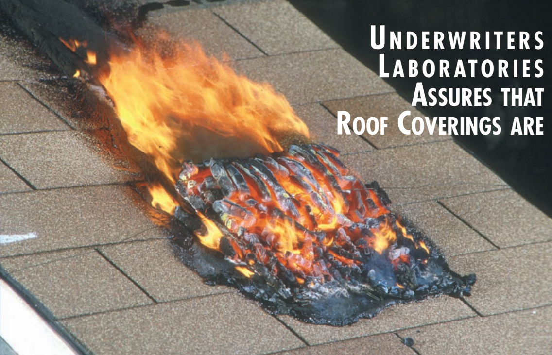
Figure 1 - UL provides conformity assessment programs with respect to fire, wind and uplift testing of roofing materials.
