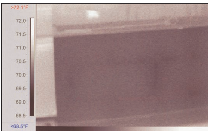
Figures 4 (left) and 5 (right) are thermograms showing water intrusion and are the interior wall of Figures 2 and 3. Water intrusion was extensive at this facility. The anticipated repair procedures and cost will exceed $1.2 million.
