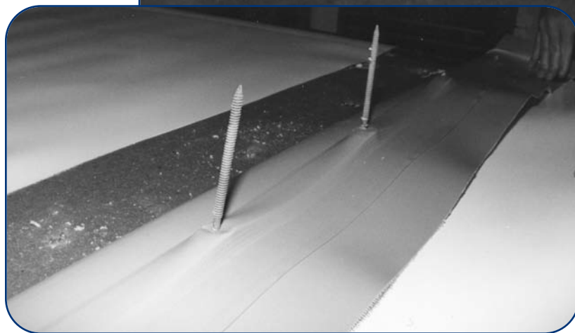
Figure 5. Failure modes of mechanically-attached TPO roofing systems after dynamic testing. Top photo: Membrane tearing failure mode of the system with one-sided weld. Bottom photo: Fasteners pullout failure mode of the system with double-sided weld.
