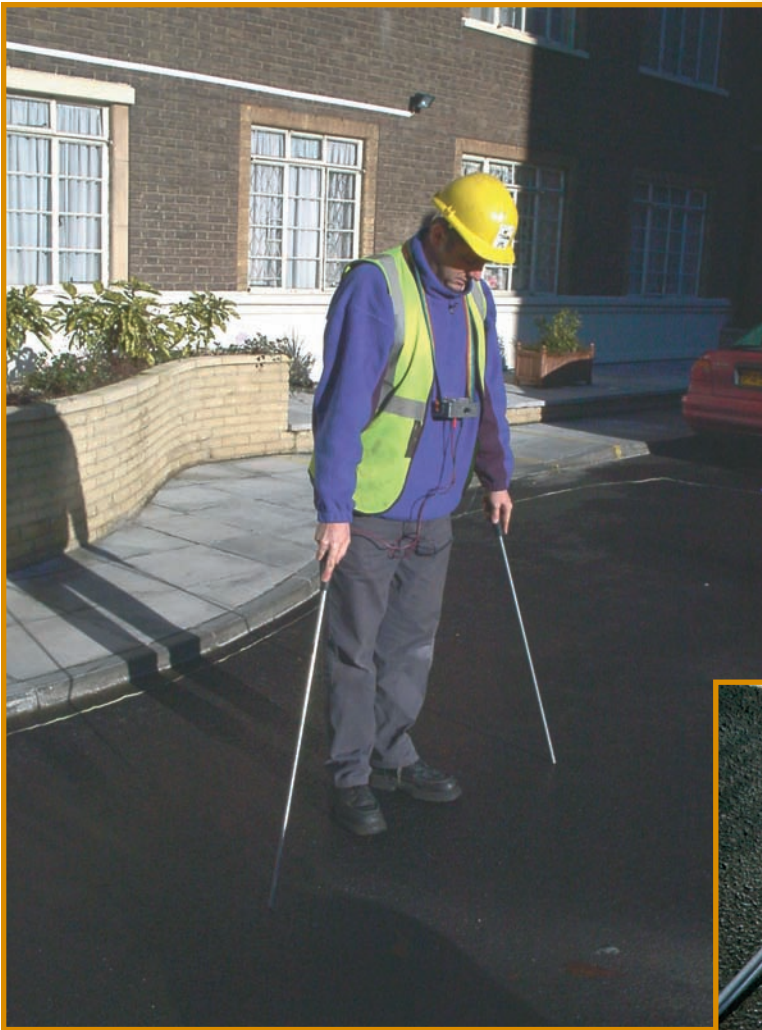
Above: Conducting the test with surface probes connected to the detector unit worn around the neck of the test engineer.
