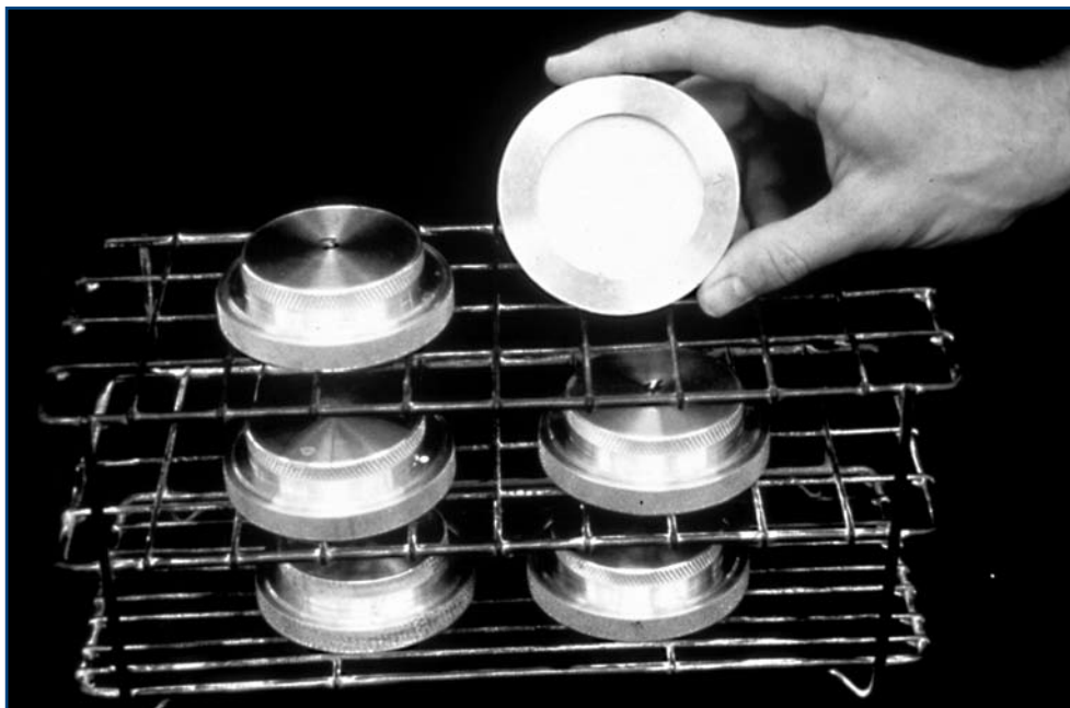
Figure 2 shows a different type of cup placed in the inverted position on a wire grid to allow air to pass freely underneath the membrane. After several hours to achieve equilibrium, the cup is weighed, and a plot of cup weight versus time is generated.
