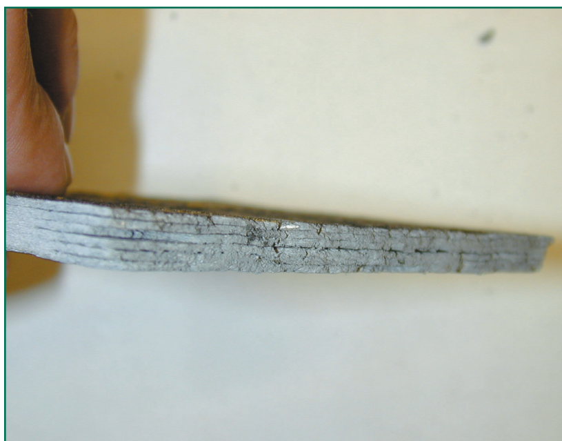
Photo 5 – Cohesive failure of the laminates
