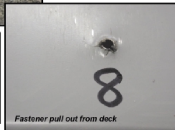
Figure 6: Wind uplift performance of single-ply, mechanically attached system.
