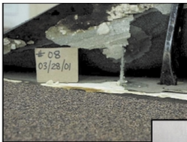
Figure 6: Wind uplift performance of single-ply, mechanically attached system.
