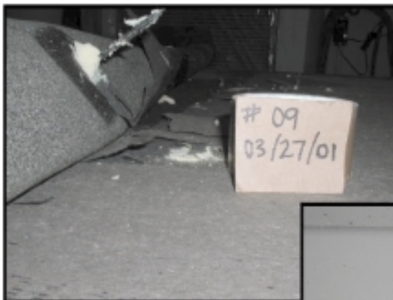
Figure 5: Static wind uplift performance of single-ply, mechanically-attached system.
