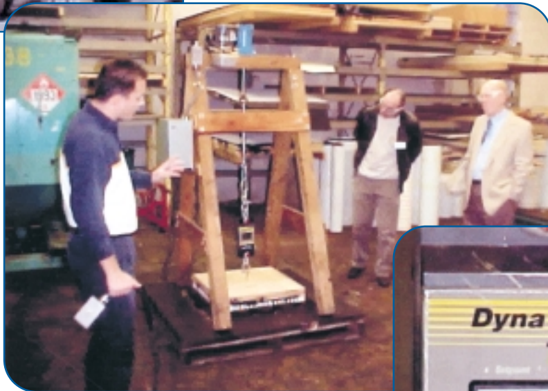
Photo 6: FM 1-52 Field Pull Test.
