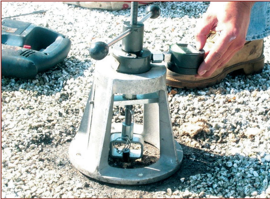
An example of a pullout tester as described in FX-1. Photo courtesy of Olympic Fasteners.
