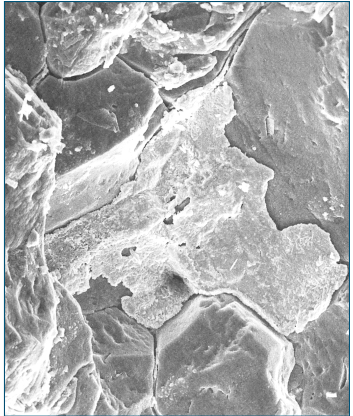
Figure 3 - Microscopic view of marble.
