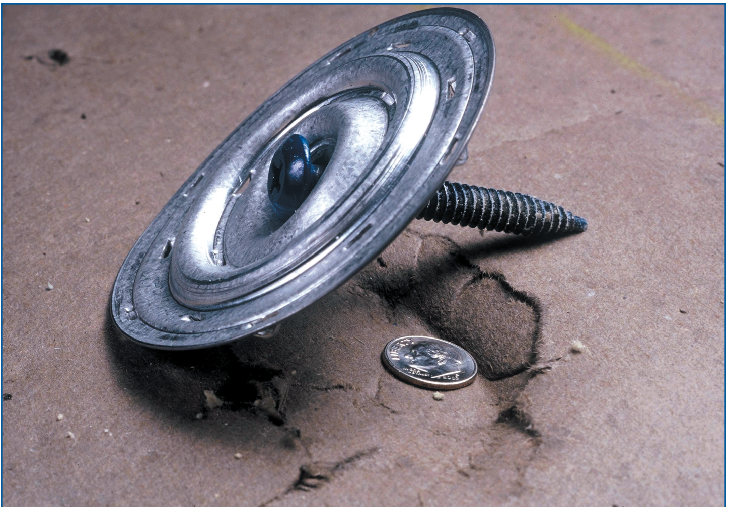
Photo 5: Damage to insulation.
