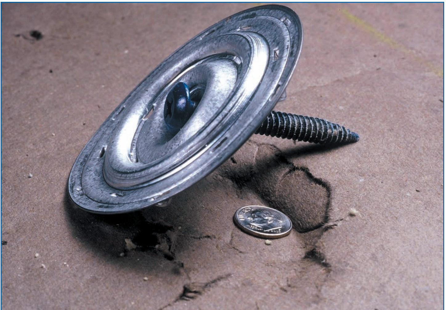
Photo 5: Damage to insulation.
