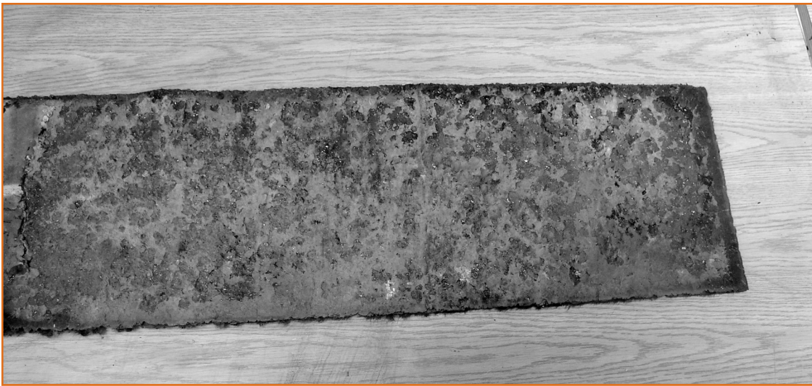
Figure 2: Felt lap sample gravel and flood coat removed.
