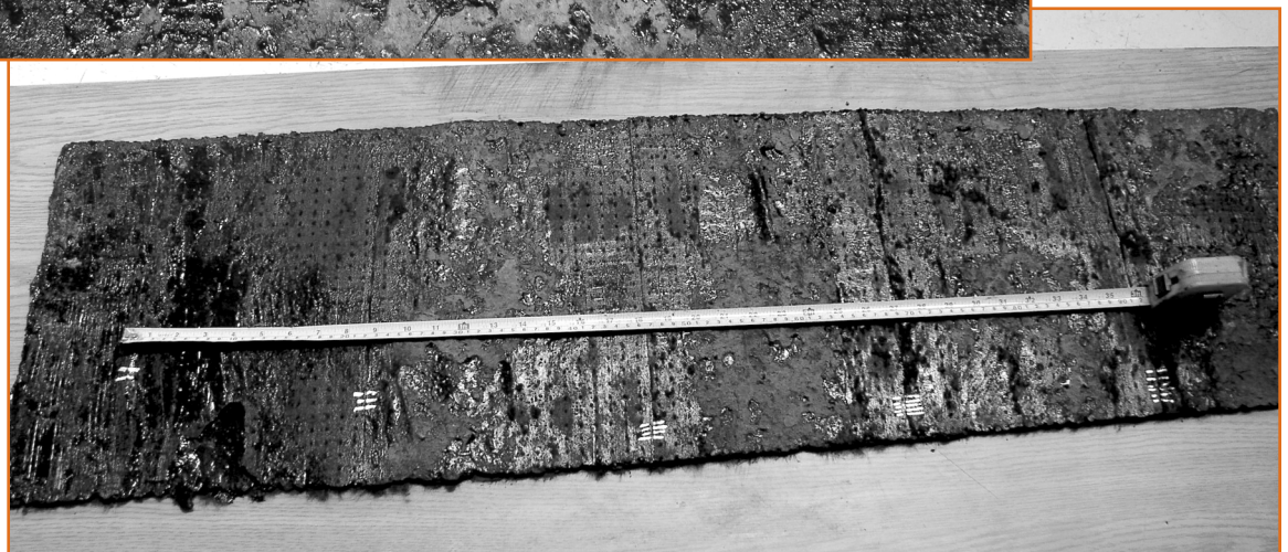
Figure 6: Measuring felt exposure.
