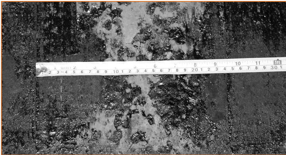
Figure 5: Felt exposure of 9.5 inches.
