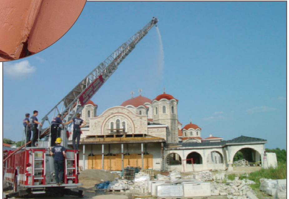
Below: Figure 14 - Water testing of the outer dome surfaces using fire fighting apparatus. The nozzle at the top of the ladder delivered 1000 gallons of water per minute.
