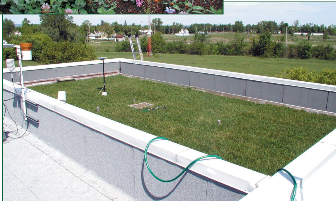
Below: Figure 4 – The sod two weeks after installation (2002). Note that the median divider separates the green roof (right) and the reference roof (left). The weather station is located at the median divider.
