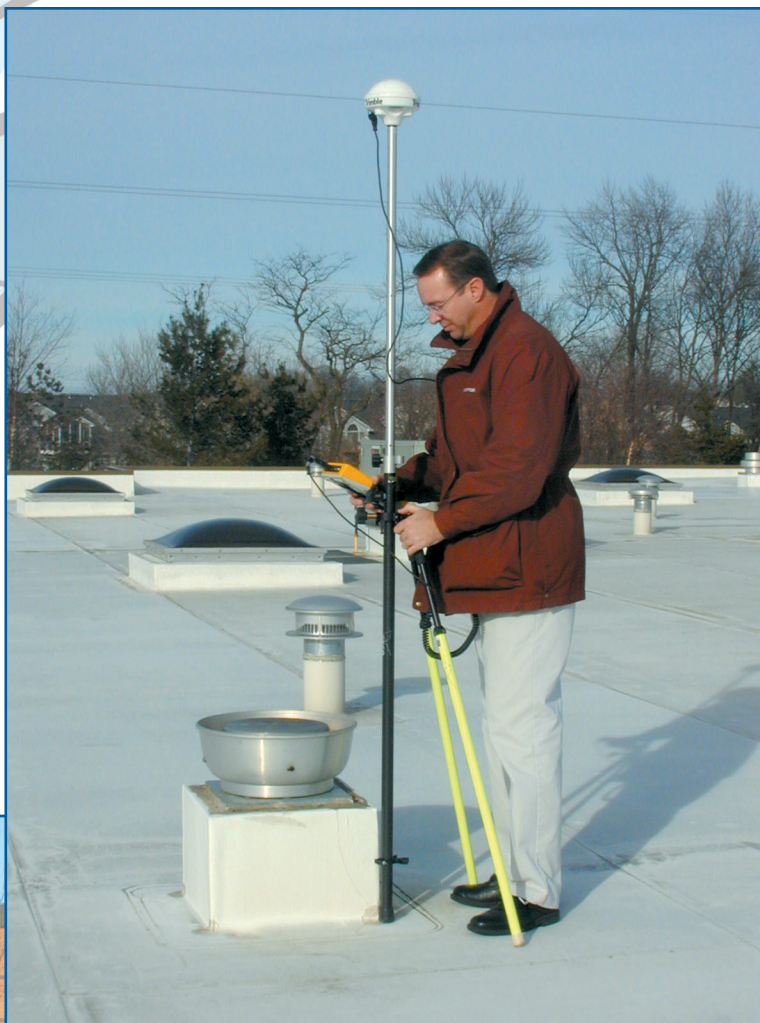
Above: GPS unit collecting data to generate a roof plan.
