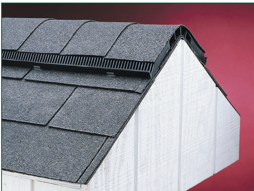
Shown is a filtered shingle-over-ridge vent (ShingleVent® II) that provides 18 square inches of net free ventilation area per linear foot. This product's external baffle system deflects wind up and over the ridge, creating low pressure above the vent openings on both sides of the vent that literally lifts or pulls air evenly out of the attic.
