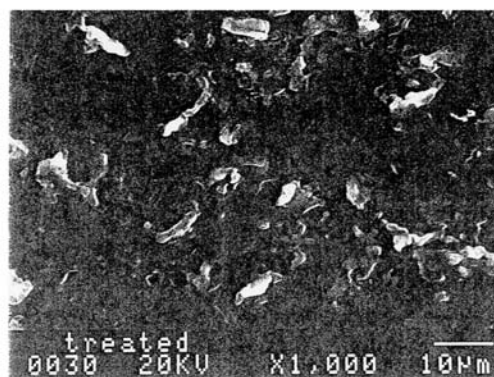
Figures 3 and 4: Microphotographs of treated and untreated new EPDM membranes.
