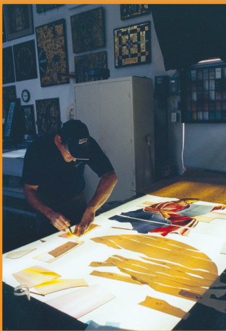
A CSS artist cuts glass on a light table, guided by the pattern piece beneath.
