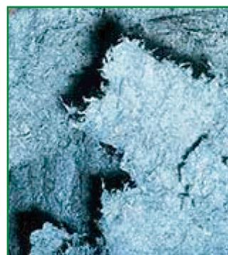
Photo 5: Processed blue asbestos (Crocidolite).
