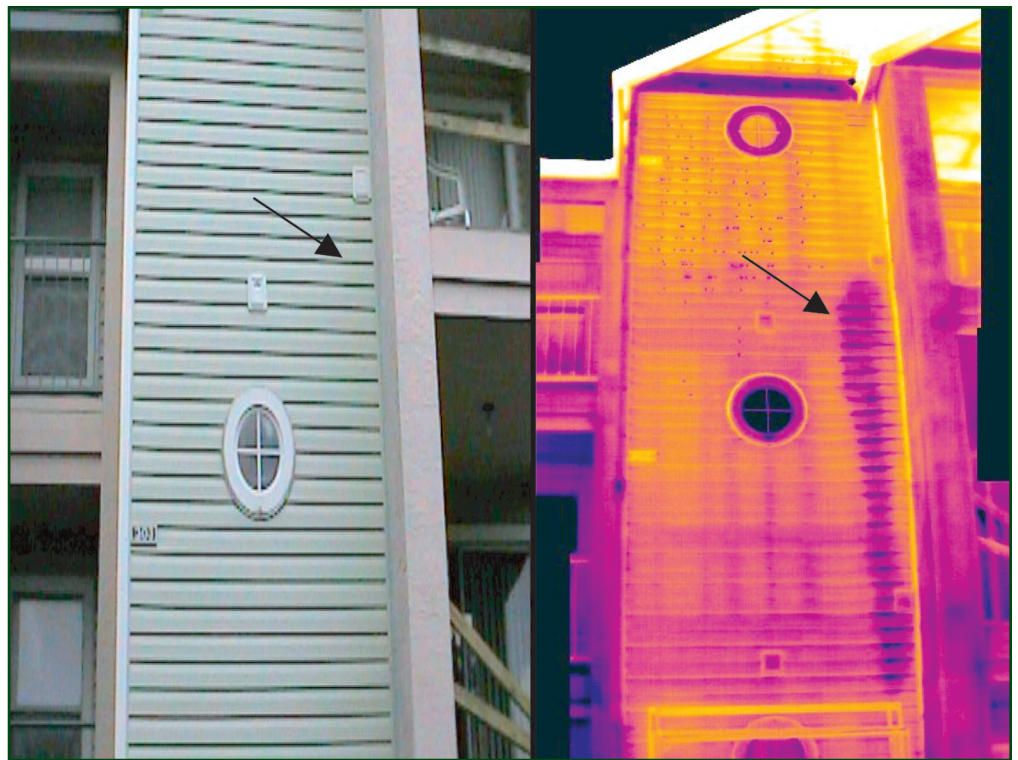
Photo 2 (left) shows apparently well-constructed exterior wall. Photo 3 (right), using an infrared camera, shows moisture infiltration not detected by the naked eye.
