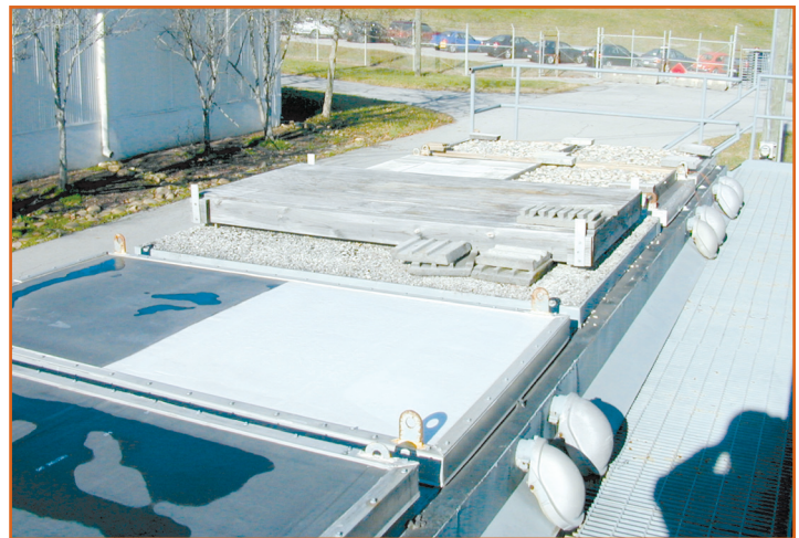
Figure 2: Test sections configured for the ballast test.
