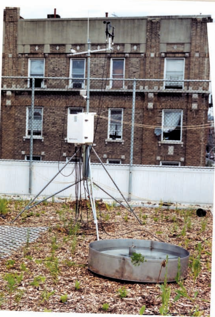
Weather station instrumentation with precipitation collection and thermo-couples set throughout the system.
