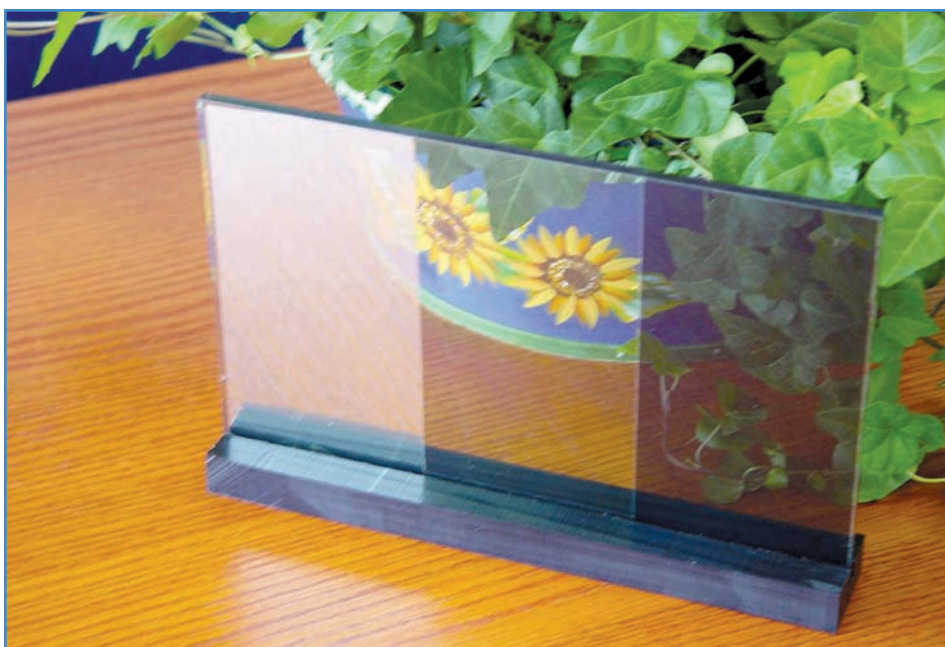
Photo 1: Conventional reflective window film (left), V-Kool clear spectrally selective film (center), and conventional tinted film (right).
