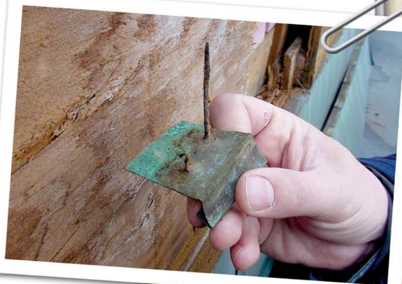
Photo 7 (above): Corroded copper fastener.
