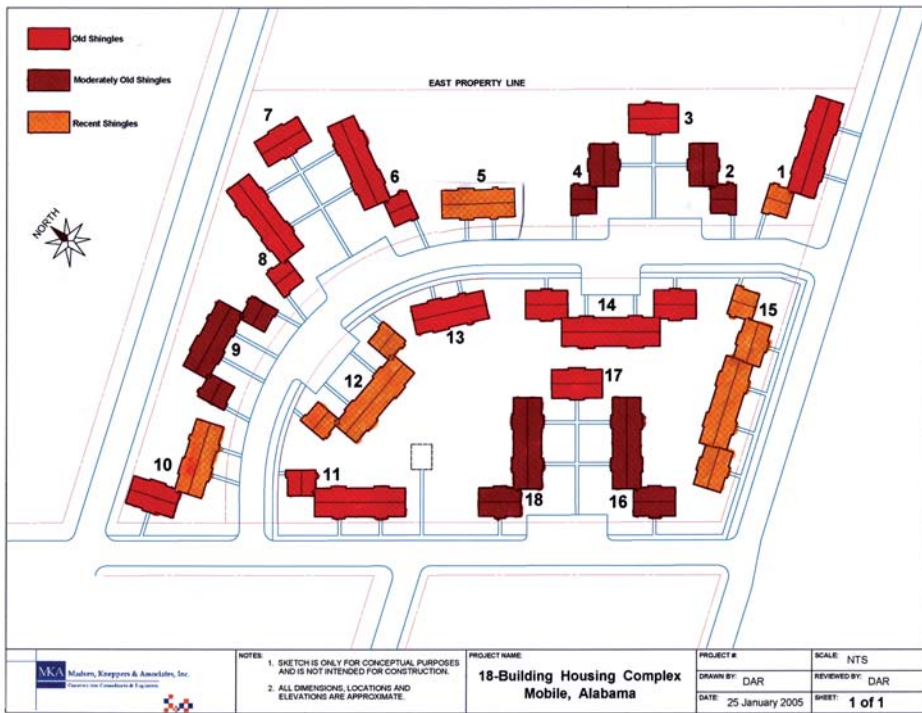
Figure 1 – The “old,” “moderately old,” and “recent” shingle roofs were each widely distributed throughout the housing complex, as can be seen with the project site plan.
