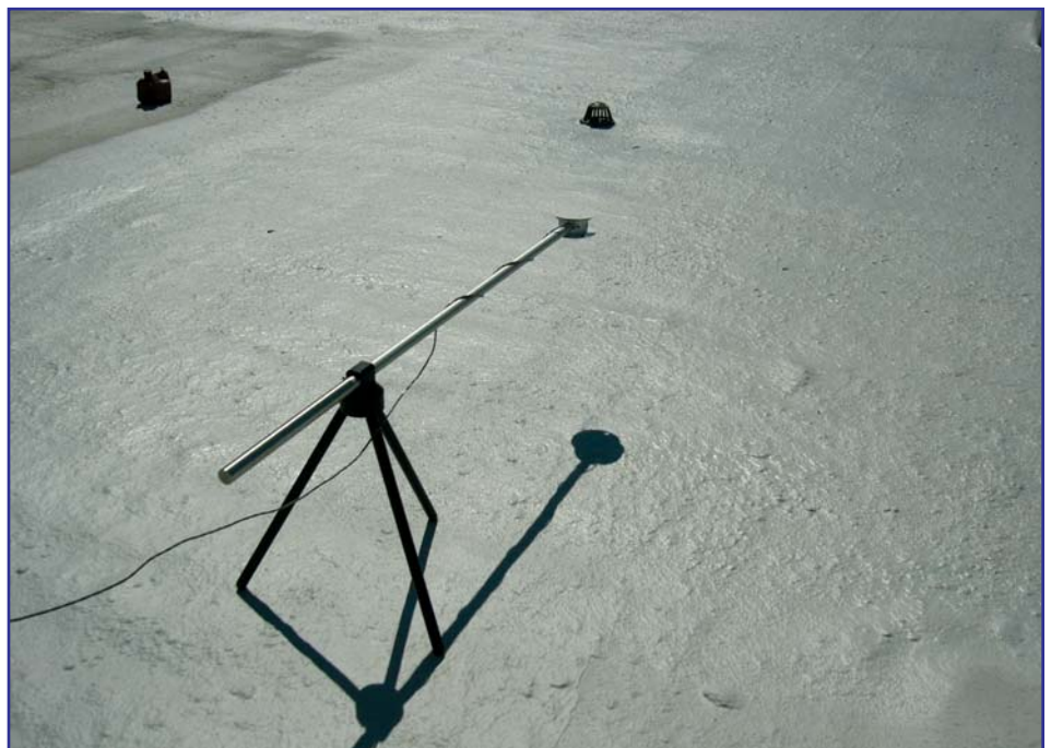
Figure 1 – Albedometer measuring foam roof reflectivity.
