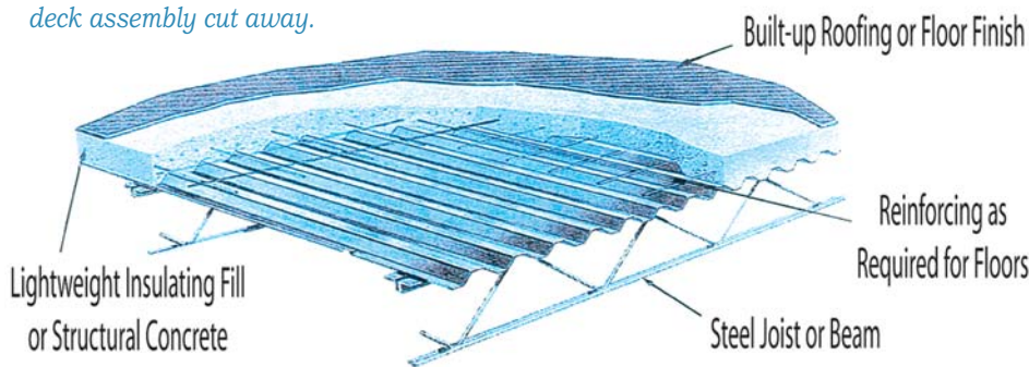
Figure 2: Roofing over concrete deck assembly cut away.
