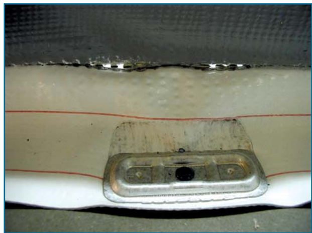
Dynamic test – Wind uplift rating 60 psf.
