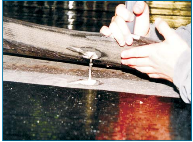
Dynamic test – Wind uplift rating 75 psf.
