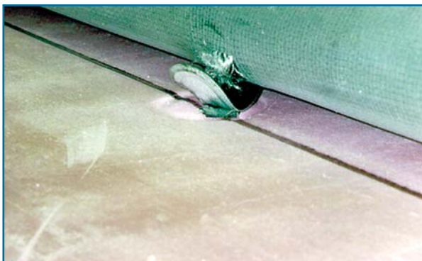
Static test – Wind uplift rating 90 psf.
