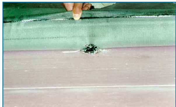
Dynamic test – Wind uplift rating 45 psf.
