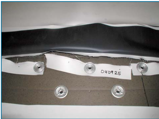
Static test – Wind uplift rating 135 psf.
