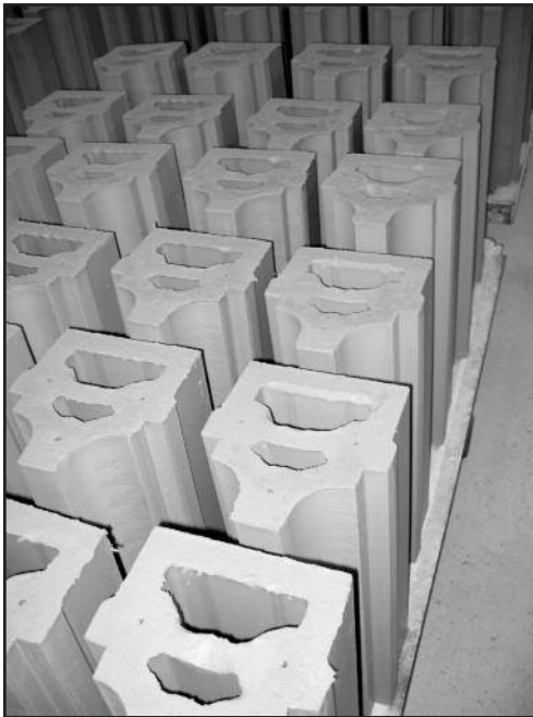
Figures 9A and 9B – New terra cotta was manufactured by extrusion and hand pressing.
