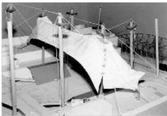
A working physical model helped develop and test installation procedures.
