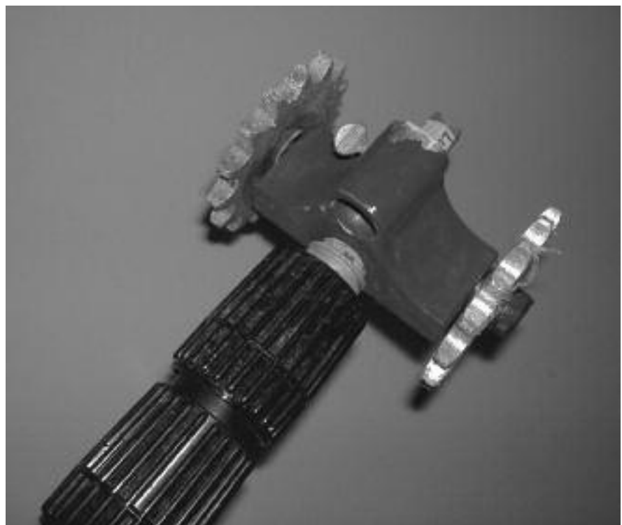
Sounding tool attached to pole. Teeth on gears tap on concrete. As tool rolls over spalled areas, the sound changes.
