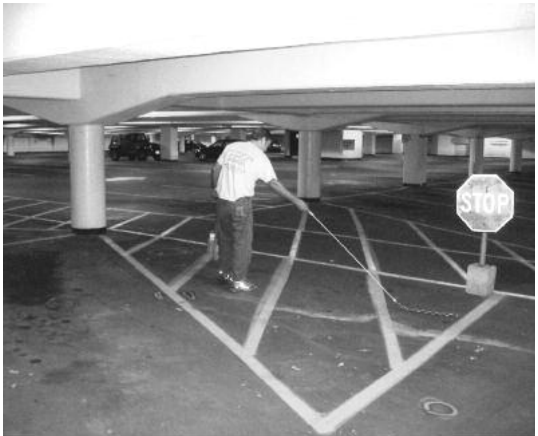
Chain Dragging. When the chain drags over a spall, a distinct hollow sound is heard. Spray-painted areas indicate spalls.
