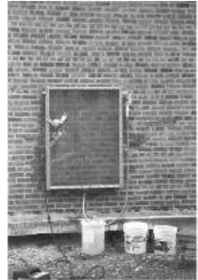
Figure 8 – Water penetration test in progress.
