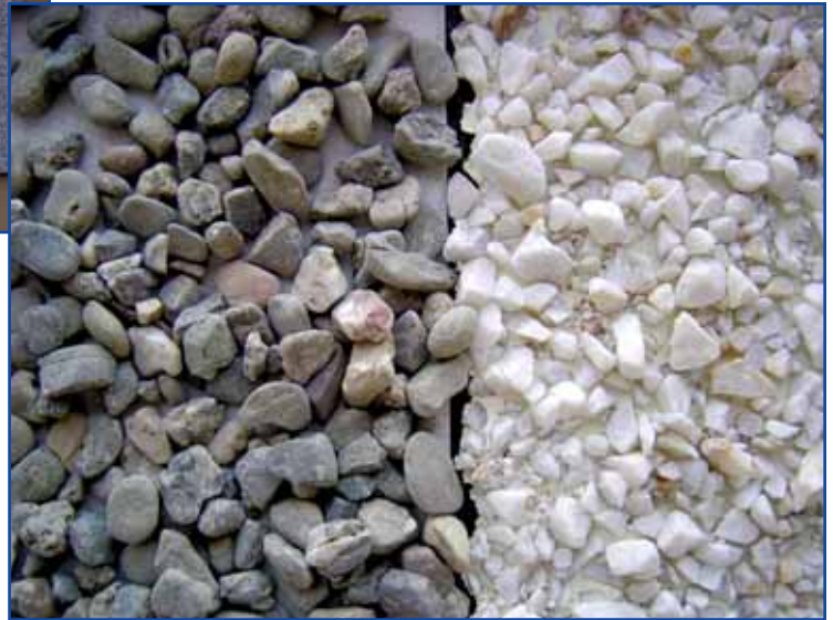
Photo 3 – Conventional (left) and Title 24-compliant aggregate (right).
