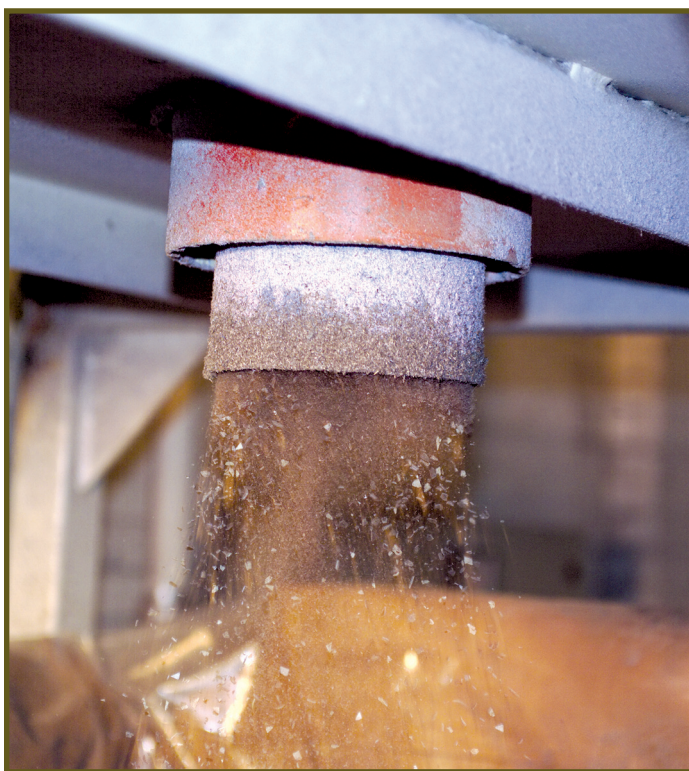
Figure 7 – PVC membrane being ground for recycling.
