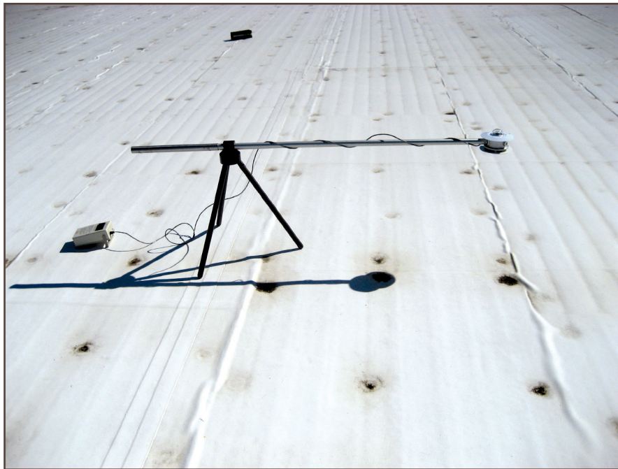
Photo 2 – EPDM in Minnesota, 1.5 years old, acrylic coating.
