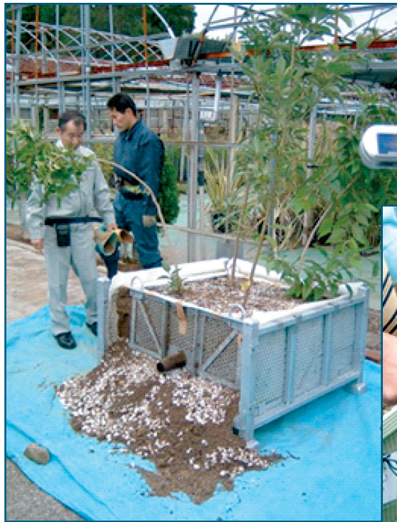
Photo 1 – Root-penetration test for trees. (One side panel is removed for inspection of root penetration.)
