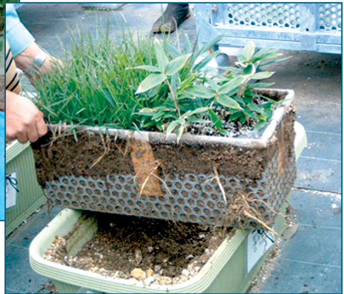
Photo 2 – Root-penetration test for plants. (An inside container is dug up for inspection of root penetration.)
