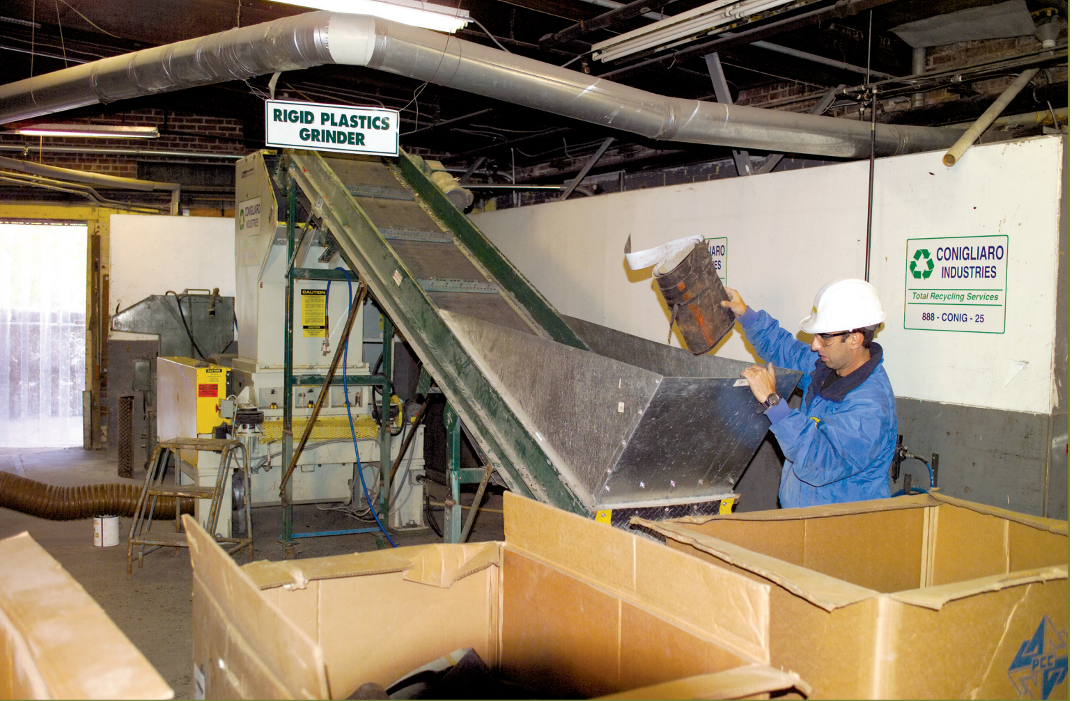
Recyclers use specialized grinding equipment to convert retired vinyl membrane to chunks or a powder. Image courtesy Vinyl Roofing Division, CFFA.
