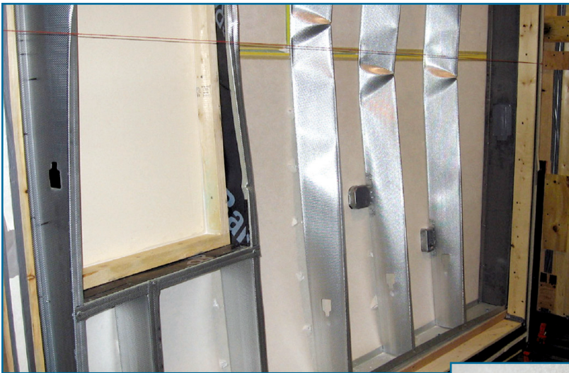
Figures 5A and 5B – The air barrier systems tested by Intertek withstood wind gusts equivalent to 168 mph, remaining fully adhered and intact while the substructure was brought to failure.
