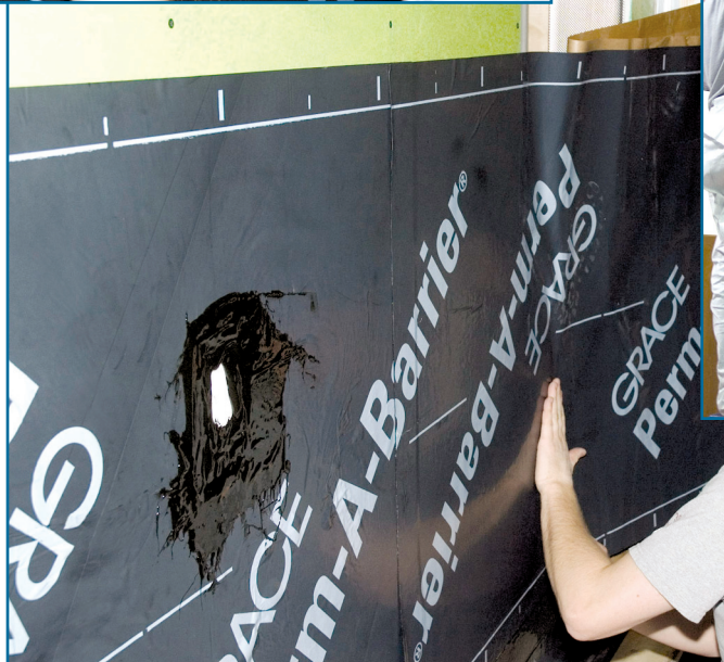
Figures 4A, 4B, and 4C – Photographs of some of the six wall specimens tested by Intertek. Each wall specimen was constructed according to ASTM E 2357 specifications, with one of the three air-barrier materials tested.
