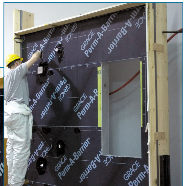
Figures 4A, 4B, and 4C – Photographs of some of the six wall specimens tested by Intertek. Each wall specimen was constructed according to ASTM E 2357 specifications, with one of the three air-barrier materials tested.
